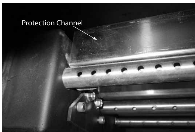
Figure 4.11 Reinstall Baffle Protection Channel
